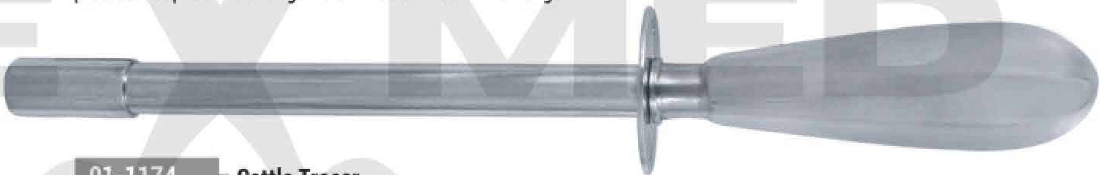
01-1174 Cattle Trocar This cattle trocar is used to relieve bloating. Complete with cannula, a hollow tube which remains when trocar is withdrawn to allow gas to escape. Stainless point. Metal handle 9.5" L. Tube is 5-1/2" L. 3/8" I.D.
