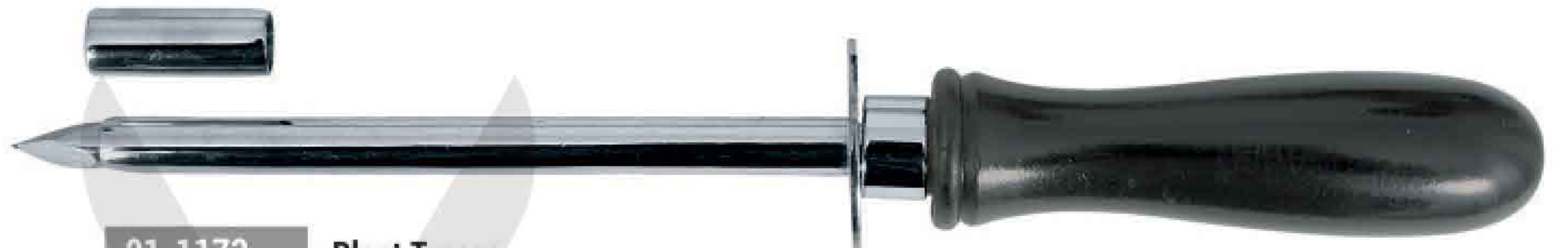
01-1173 Bloat Trocar The flat-to-round shape has made this wooden-handled trocar very popular for venting animal gas accumulations. Includes stainless steel cannula and protector cap. Cannula length is 6". Also available in 5" length.
